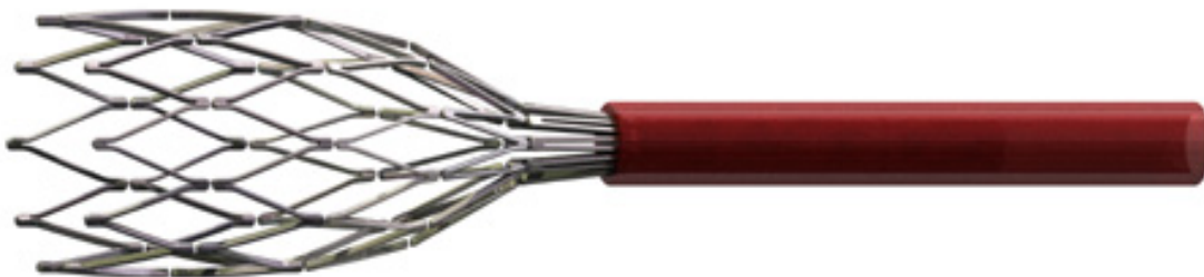
Fig. 2.5 NiTi stent self expands after being removed from endoscopic installation tube [13]
