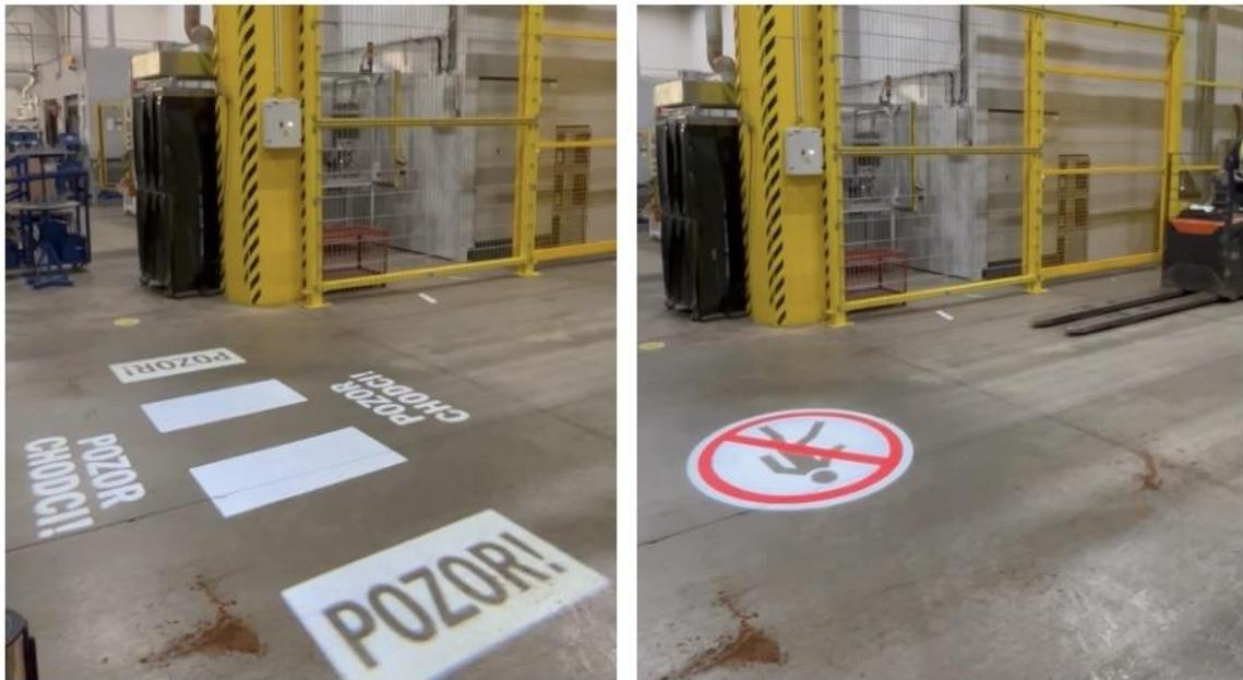
*Figure 9: Crossing projection device*
