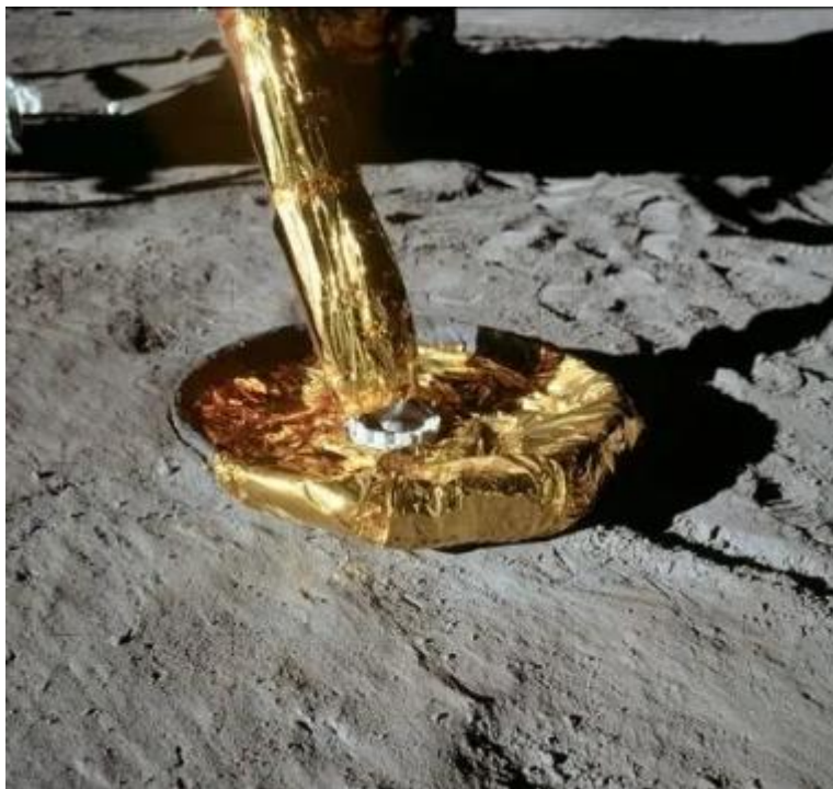
Figure 3-3 Kapton wrapped around the leg of the lunar module while standing on Moon's surface [11]
