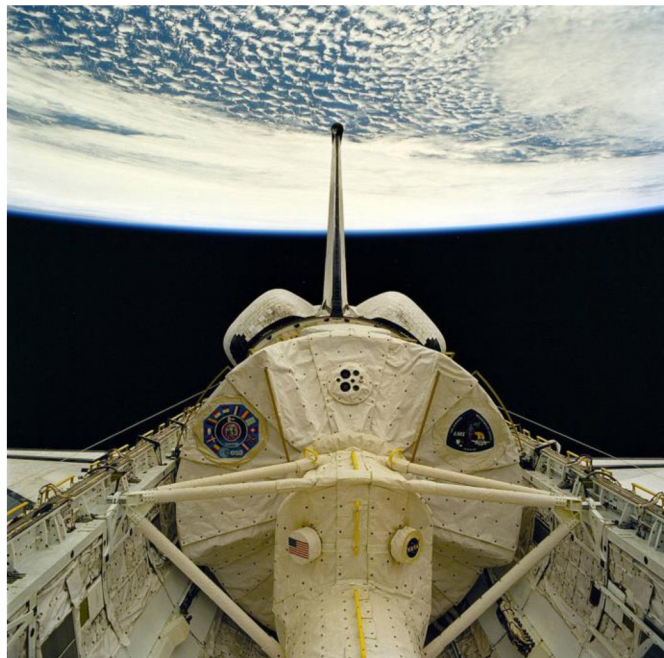
Figure 3-2 Beta Cloth used as an outer cover Atlantis Space Shuttle
