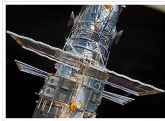
Figure 3-4 Hubble Telescope covered in Teflon [14]
