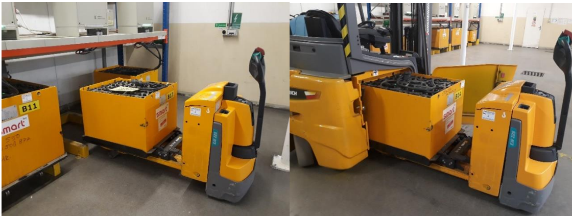
Figure 16: Battery changing process
