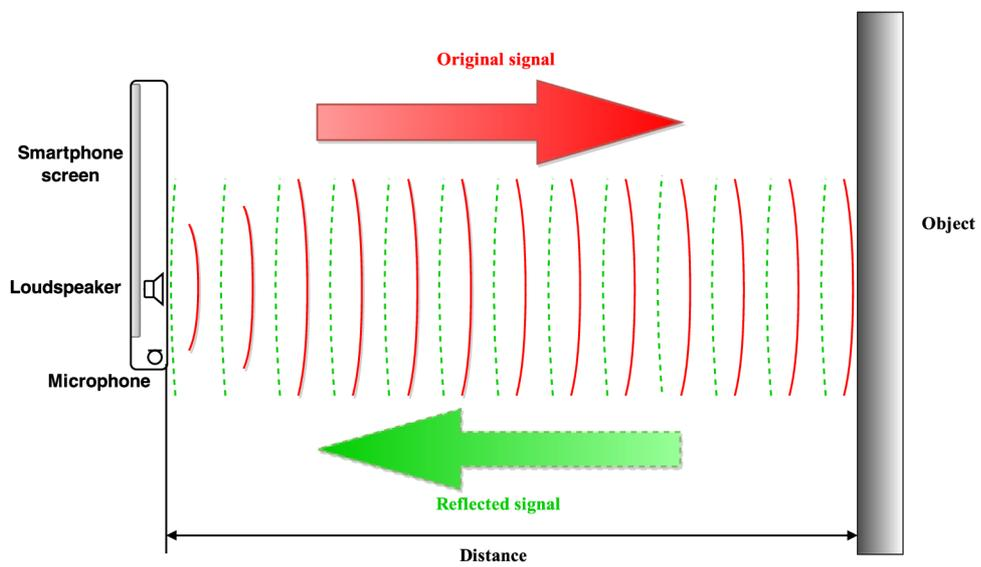
Figure 2.2: Smartphone used as sonar with usually placed components.
