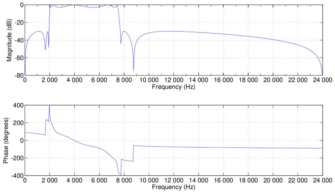
Figure 4.10: Magnitude and phase response of band-pass filter.
