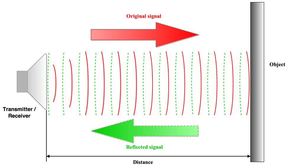
Figure 2.1: Principle of sonar.
