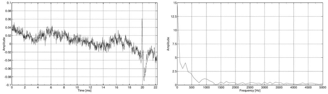
Figure A.3: Recorded signal 220 Hz and its spectrum.
