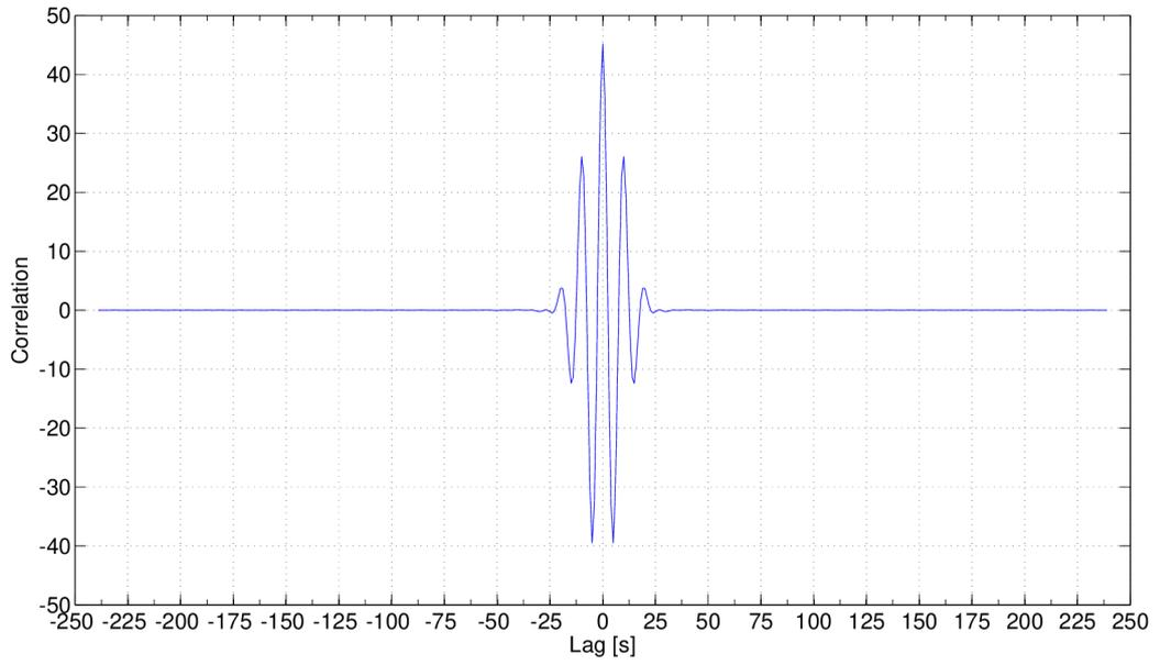
Figure 4.7: Autocorrelation of chirp wave from 4.6.
