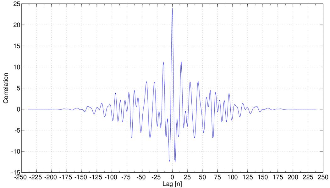
Figure 4.12: Autocorrelation of filtered white noise wave from 4.11.
