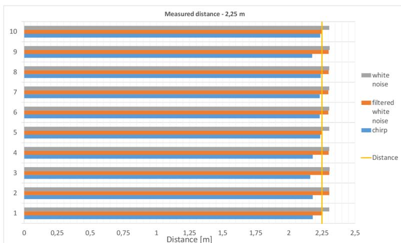
Figure B.11: Measurement of 2.25 meters.
