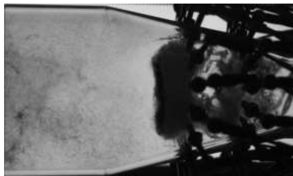
Figure 170 Cavitating vortex ring passing through the measuring plane P2
