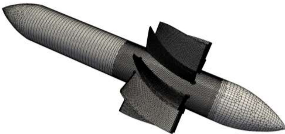
Figure 121 Surface mesh of the swirl generator - CG2
