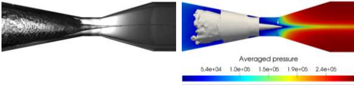
Figure 131 Main flaws of the numerical analysis of the cavitating flow considering the full geometry of the test section (CG1) – overpredicted cavitation of the boundary layer and absence of the cavitating vortex filament downstream the spike of SG. (75% of the vapor)
