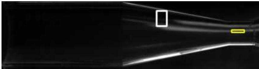
Figure 44 Regions of interest which were utilized for the spectral analysis of pixel intensity fluctuations. Yellow – ROI 1, White – ROI 2
