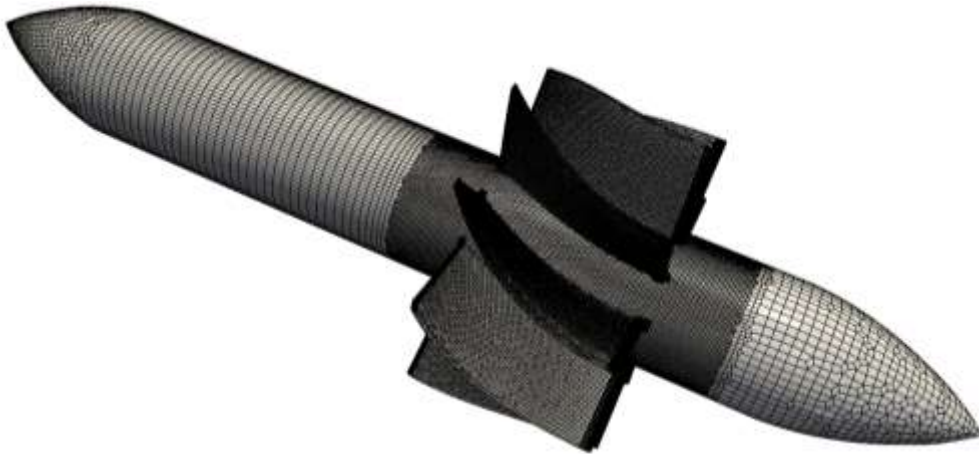
Figure 120 Surface mesh of the swirl generator - CG1
