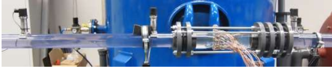
Figure 168 Venturi nozzle mounted to the test rig
