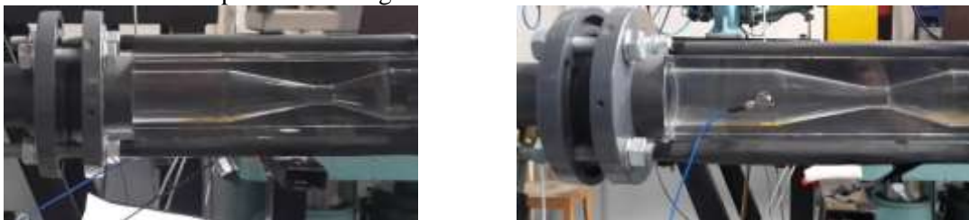
Figure 17 Position of the accelerometer during the measurement of the eigenfrequency of the test bench in vertical (left) and horizontal direction(right).
