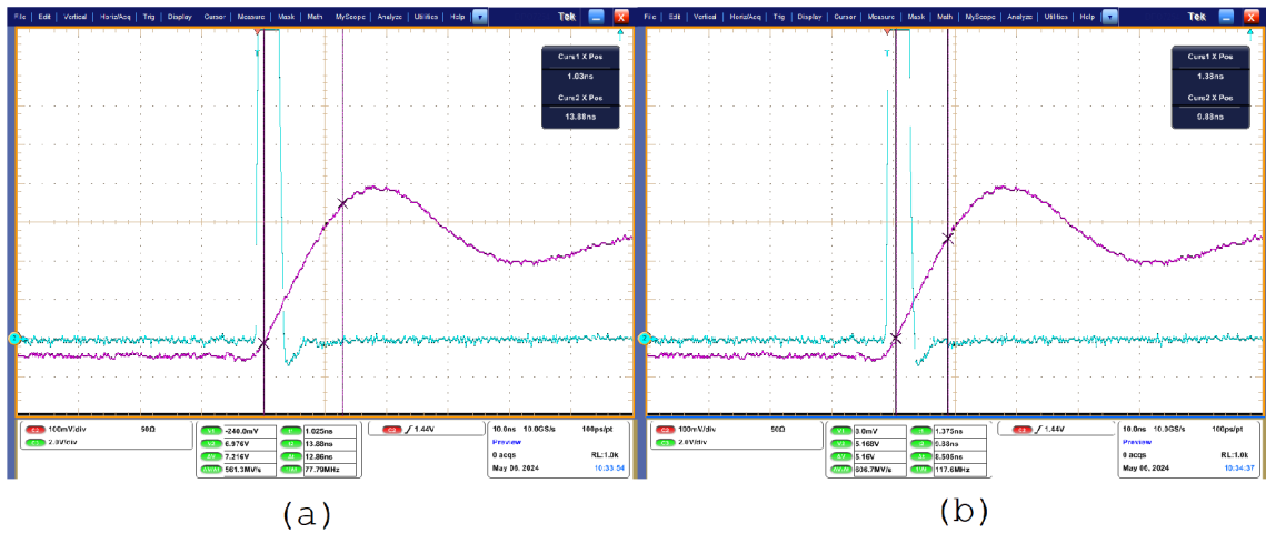
Fig. 4.7: Driver output waveform: (a) 50\ \Omega load; (b) PSN as the load
