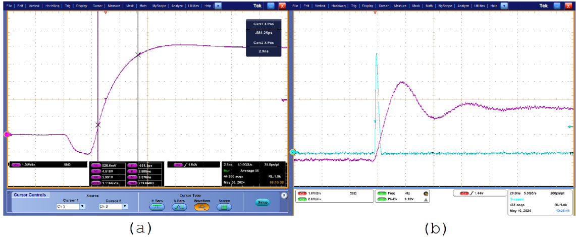
Fig. 4.6: Driver output waveform: (a) 50 Ω load; (b) PSN as the load
