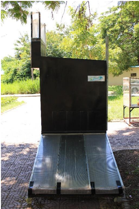
Figure 12: Solar hybrid dryer (photo: Ana Hubackova)
