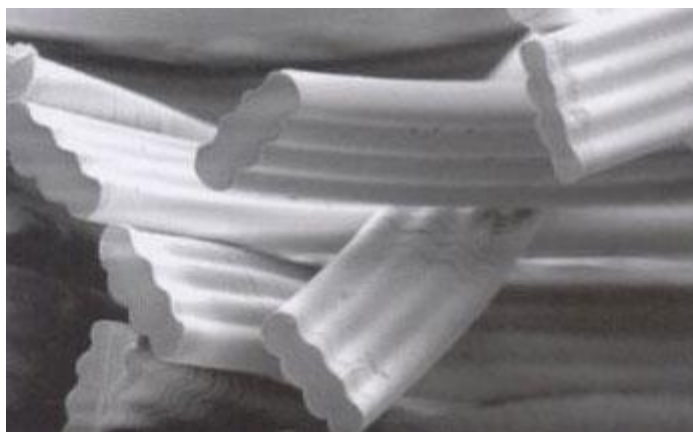
Obr. 7 Vláknó CoolMax Extreme Hexachannel [22]
