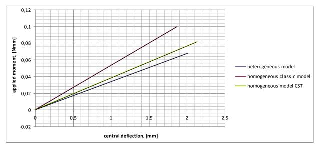
**Fig. 5.10.** Comparison of FE simulations of 4-point bending using different constitutive models for the case of fibre declination angle of 30 degrees.
