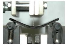
**Fig. 3.2.** Bending test of fibre composite with rubber matrix
