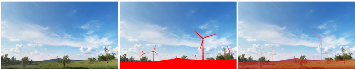
Fig. 86: Demonstrating how to use natural features to place a render on a photo and how accurate this method is in making 3D model of the real terrain
