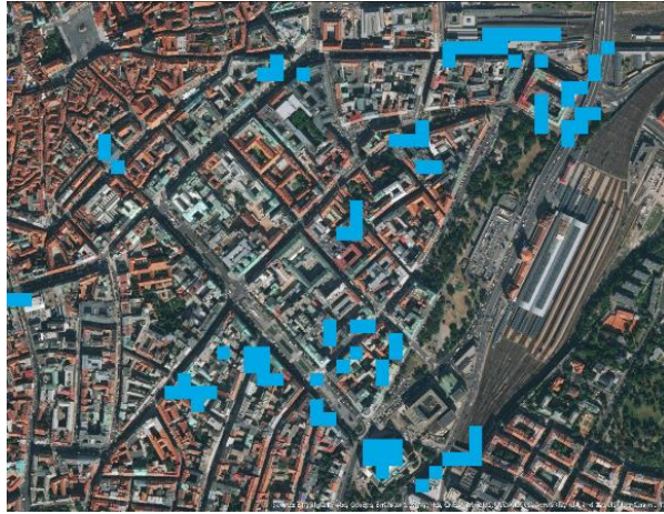
Figure 5a. Clouds incorrectly classified as water in a highly urbanised area, surrounding Prague main railway station. Globeland30. Source: Author.
