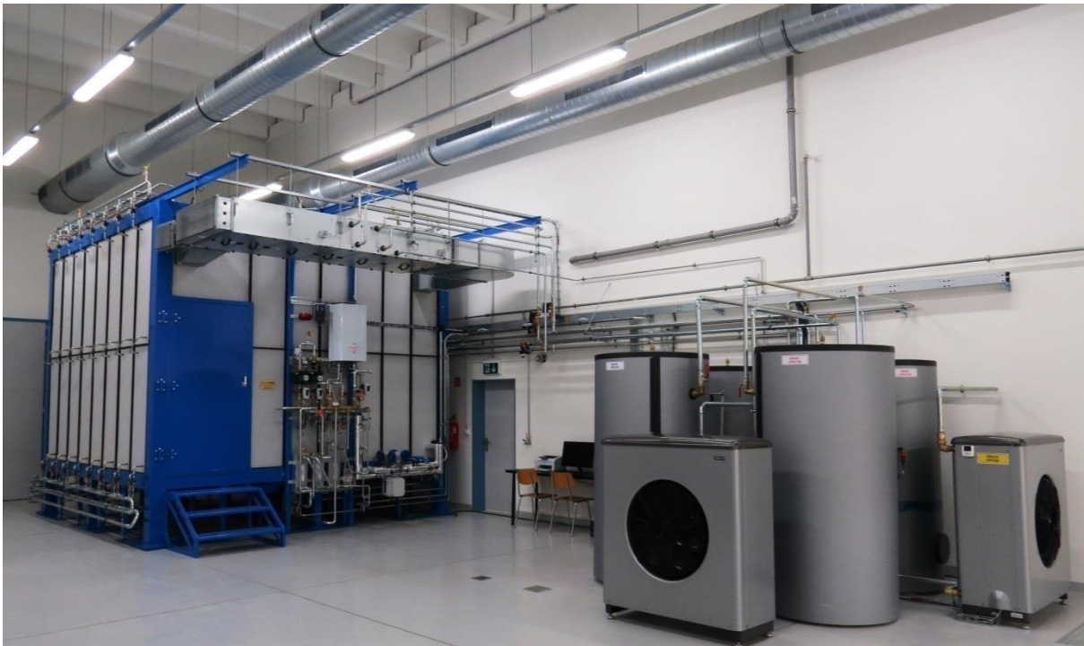
Fig. 26 HeatLab calorimetric chamber for heating/cooling equipment testing
