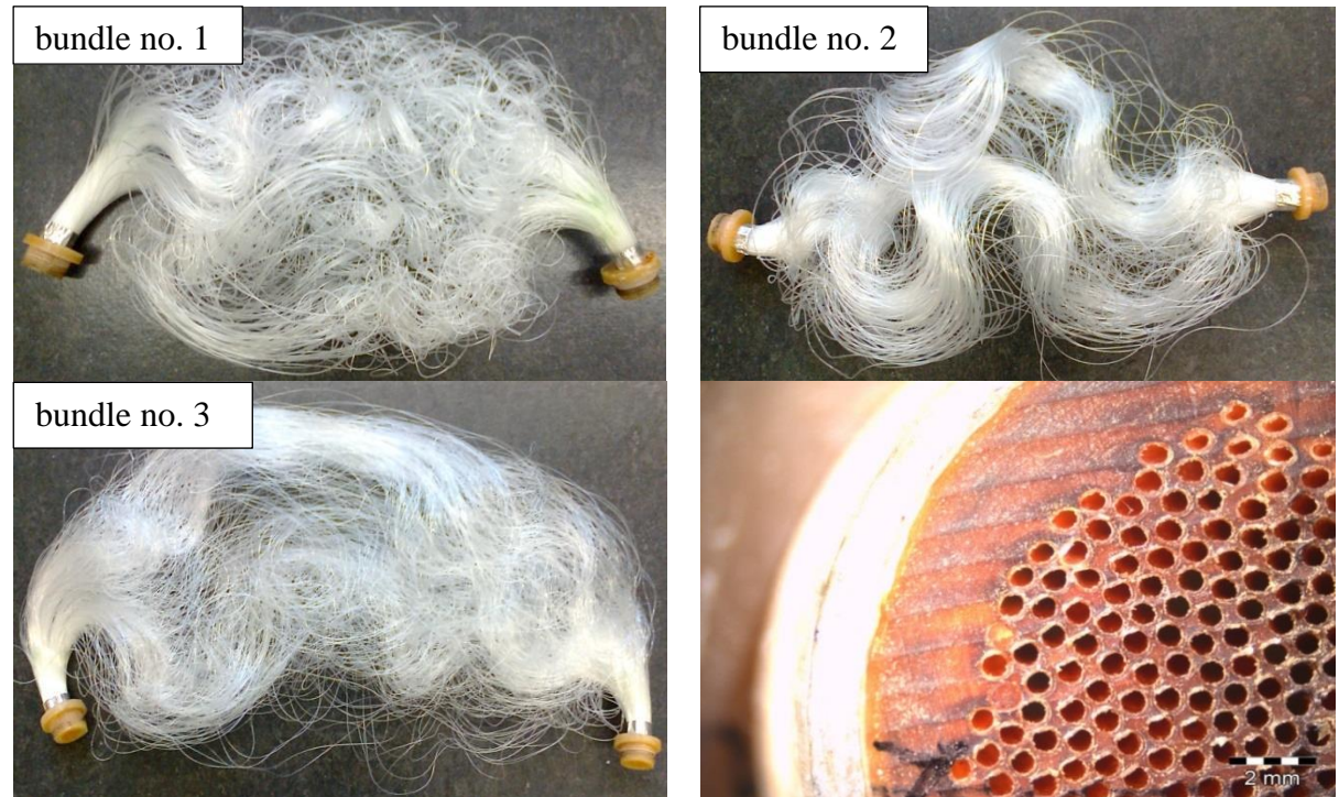
Fig. 19 Tested hollow fiber bundles and quarter of the cross section of bundle no. 1.
