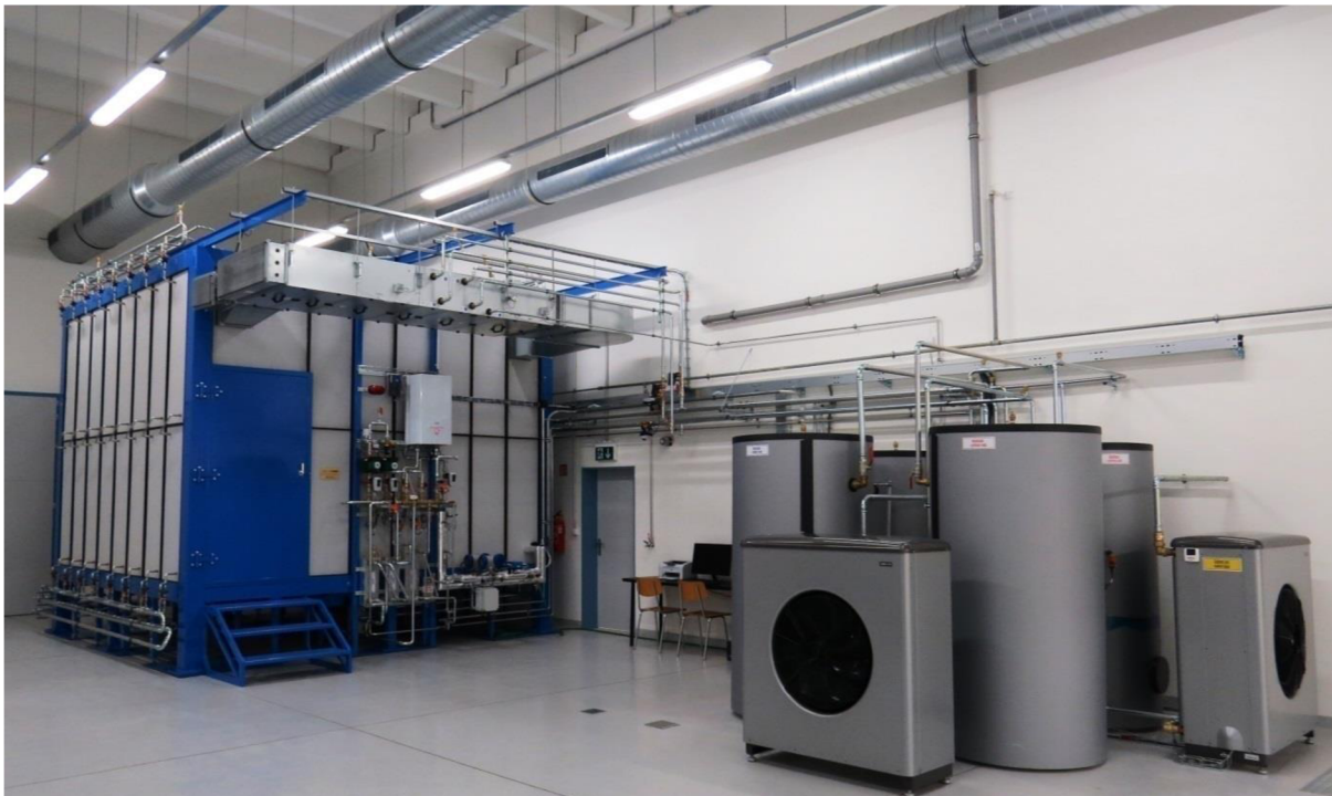
Fig. 26 HeatLab calorimetric chamber for heating/cooling equipment testing
