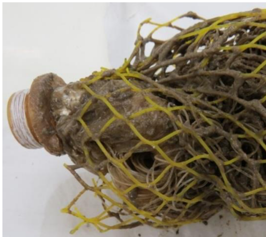
Fig. 44 Heat exchange bundle no. 2 after 35-day experiment with laundry wastewater no. 2 (left) and fouling evolution in time: OHTC (black squares) and fouling thermal resistance (white squares).
