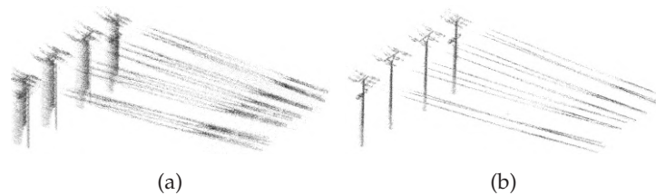
Figure 7.25: Example of ambiguities caused by reconstruction errors (a), which disqualifies the model to be used for practical measurements. We obtained such results when we used only poses provided by GNSS/INS subsystem without any refinements by SLAM or point cloud registration. Our solution (including SLAM) provides valid reconstructions (b), where both towers and wires (in this case) can be distinguished.
