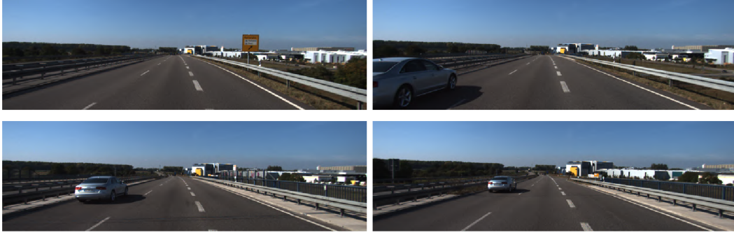
Figure 5.9: Images from KITTI data sequence #1 where GICP approach fails but our method preserves accuracy. Images show the challenging situation when over-turning car appear as confusing landmarks on otherwise empty highway.
