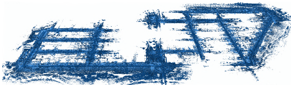
Figure 6.1: Example of LiDAR point clouds registered by CNN estimated odometry. Sequence 08 of KITTI dataset [28] is presented with rotations provided by IMU.
