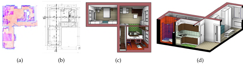
Figure 2.2: Top view of the laser point cloud (a), the footprint of the flat generated from this scan (b) and the 3D models for visualization (c), (d).
