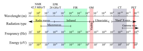
Fig. 2: Schematic image showing basic spectroscopic methods with the frequencies, wavelength and corresponding energy ranges where the methods operate.
