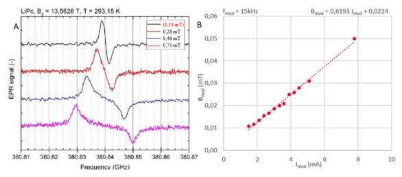
Fig. 5.3: A) Overmodulated ESR spectra of LiPC obtained during modulation coil calibration. The spectrum has to be overmodulated to allow determining the modulation amplitude. The black line corresponds to the case when the spectrum is not overmodulated enough to determine the modulation amplitude directly. However, it can be re-calculated from the calibration curve (value in brackets in legend). B) Field Modulation amplitude as a function of AC current in the coil and its linear fit.
