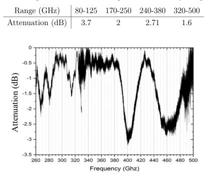
Fig. 4.23: Normalized overall double-pass attenuation of EPR probe measured by VNA without window. The reference data were taken with the mirror placed on the probe input.
