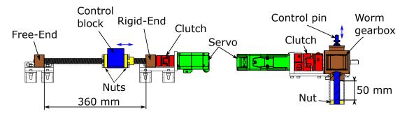
Fig. 4.17: The drawings of movement system. Left) X and y, Right) z-movement system.
