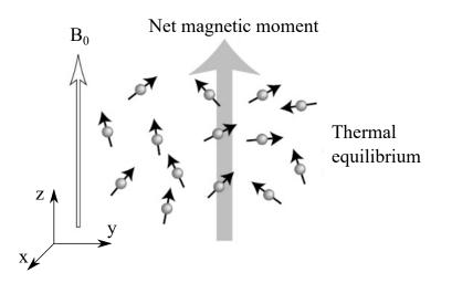
Fig. 2.8: System in thermal equilibrium after exposing to external magnetic field. Magnetization is getting bigger with the increasing external magnetic field. If the external magnetic field  $B_0$  would be equal to zero, the spin moments' sum will result in zero magnetization. Taken from [92].
