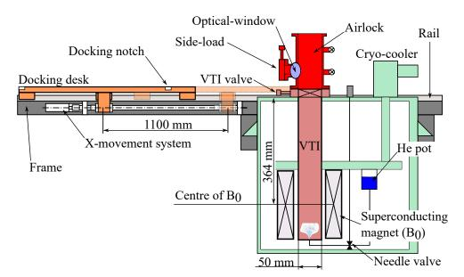
Fig. 4.4: The illustrative scheme of magnet frame.
