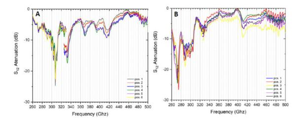
Fig. 5.12: Results from VNA measurements for invidual cells of carusel SH. A) Carusel cells share one big mirror, B) Each cell has its own mirror (diameter of 5.5 mm).
