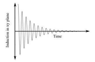
Fig. 2.12: Observable relaxation of xy magnetization  $M_{xy}$  after a pulsed excitation. The exponential decay is proportional to  $T_2$ . For the first time, it was observed in an NMR experiment by inserting a detection coil into the xy-plane [104].
