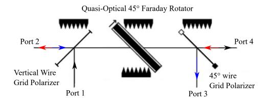
Fig. 3.9: Schematic of a QO circulator based on a Faraday rotator and two wire polarizers. A vertically polarised m.w. (red) inputs in Port 1 leaves  $-45^{\circ}$  polarised at Port 4. The m.w. reflected back, which enter Port 4 with 45° (black) polarization leave the setup in port 2. And the same m.w. which is reflected back and enters Port 2 (blue) with horizontal polarization leaves by Port 3 with  $-45^{\circ}$  polarization. Taken from [125].
