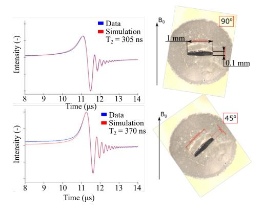
Fig. 6.6: Rapid scan measurement on LiPC with the different crystal direction to magnetic field  $B_0$ . Sample was glued to the rod of RSH by epoxy. Parameters of the measurement:  $B_0 = 5.452$  T, T = 293 K, frequency sweep 152.56 - 152.63 GHz, number of averages 2 000 000.
