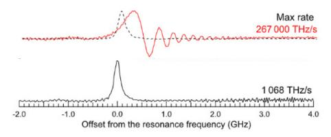
Fig. 1.2: Rapid scan spectra of the LiPc sample recorded at the fixed field of 8 T, temperature of 13 K and modulation frequencies 20 kHz and 5 MHz, and constant modulation amplitude of 8.5 GHz. In the first spectra, black, the sweep rate is not fast enough, and only absorption signal without "wiggles" is measured. Traces are labeled by the maximum sweep rate achieved at the center of sweep. Dashed curves are the deconvoluted spectra. Taken and adjusted from [28].
