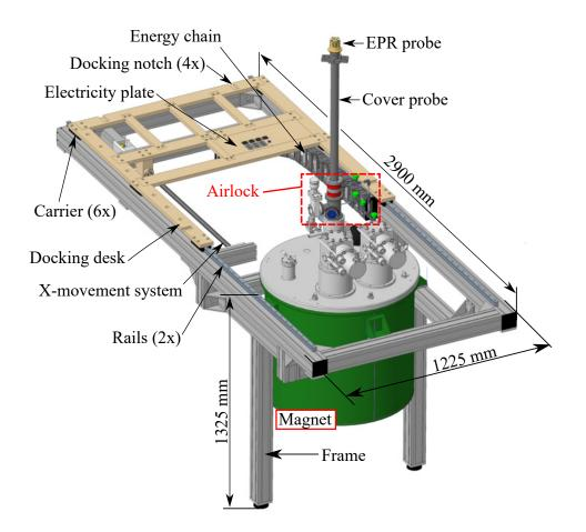
Fig. 4.6: 3D model of the magnet frame. The docking desk is in the loading/unloading position, while the EPR probe is inserted inside the airlock.
