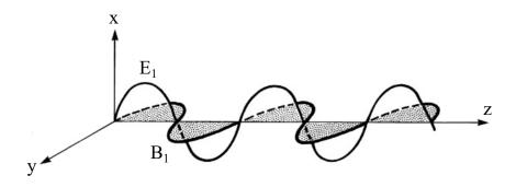
Fig. 1: Instantaneous amplitudes of electric field  $(E_1)$  and magnetic-field  $(B_1)$  components in a propagating plane-polarized and monochromatic electromagnetic beam. We note that  $E_1$  is confined to plane xz,  $B_1$  is confined to plane yz, with wave propagation along z. Taken from [6].
