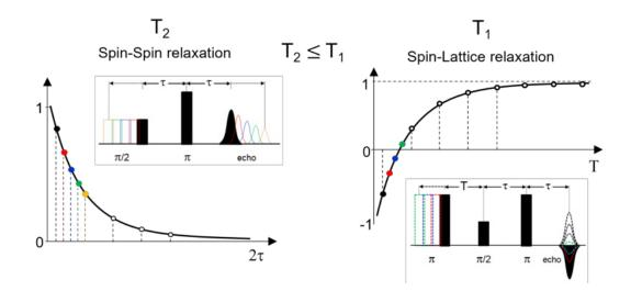
Fig. 2.13: The pulsed sequence of simple experiment for measure spin echo of  $T_2$  and  $T_1$  relaxation time.  $T_2$  represent relaxation of magnetisation in xy plane, whetever  $T_1$  represent relaxation of magnetisation in z plane. After  $\pi/2$  pulse and time period  $\tau$  always follow  $\pi$  pulse which rephase magnetisation dephasing and creates echo signal in time  $2\tau$ . Kindly provided by Dr. Petr Neugebauer.
