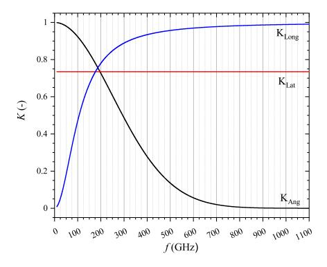
Fig. 3.6: Power distribution for different coupling errors. Parameters for calculation: beam waist  $\omega_0 = 9 \text{ mm}$ , Longitudinal displacement  $\Delta z = 150 \text{ mm}$ , Lateral displacement  $\Delta h = 5 \text{ mm}$ , Angular displacement  $\Delta \phi = 0.03 \text{ rad}$ .
