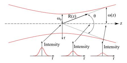
Fig. 3.3: Schematic picture of the Gaussian beam propagation with the cuts in different z positions.
