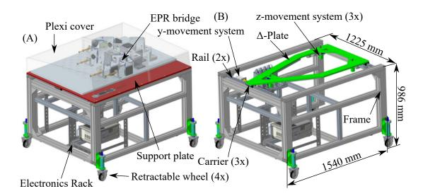
Fig. 4.11: The 3D model of EPR table. A) The model displays the EPR bridge covered by plexiglass covers. B) The model without EPR bridge, plexiglass covers and support plate.
