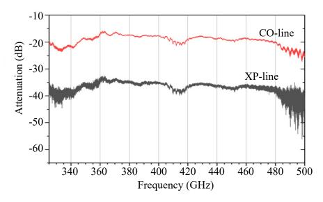
Fig. 4.13: Signal in Co and XP line with a VNA extender as RF source. The extenders were not calibrated, Therefore, there is a drop in power. Valuable information is the difference between the CO and XP lines, 20 dB.
