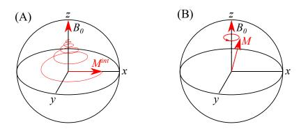
Fig. 2.9: Schematic illustration of magnetization evolution in Bloch sphere. A) Relaxation of initial magnetization  $M^{int}$  into a new position parallel to  $B_0$  field. B) Precession of Magnetization M around the  $B_0$  field. In this case, component  $M_z$ remains constant.
