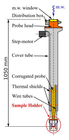
Fig. 4.20: Scheme of EPR probe.
