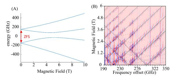
Fig. 2.5: (A)The level energy (Hamiltonian solution) of a 3/2-spin system placed into the magnet field. (B) The measurement are showing EPR map 1200x800 resolution of Mn<sub>1</sub>2Ac crystal together with simulation (dotted lines). Parameters of simulations: S = 10, g = [1.93, 1.96], D = - 13790.5 MHz,  $B_4^4 = 1.19917$  MHz,  $B_0^4$ = -0.659543 MHz. Taken from [77].
