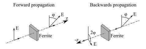
Fig. 3.7: Schematic drawing of beam propagation through Ferrite. The output of the rotation angle of polarization is independent of m.w. propagation direction. Therefore, the output of 45° ferrite rotation is for m.w. going "forward" and the same m.w. going later "backward" direction has polarization rotate by 90°.
