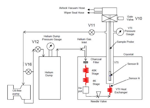
Fig. C.1: Scheme of VTI magnet
