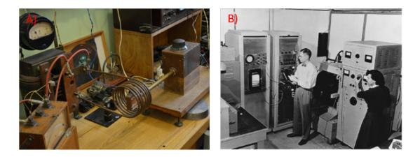
Fig. 1.1: A) First EPR Spectrometer costructed by Zavoisky. Taken from B) First commercieal 30 MHz NMR spectrometer made by R.H. Varian in 1952. Taken from [38].
