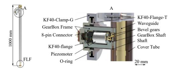
Fig. 4.21: 3D view of the EPR probe A) View of the top part of the EPR probe where the piezo step motor is located. Through shaft and set of ratio 1:1, the rotary movement is translated to FLF.
