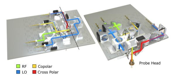
Fig. 4.15: The render of coupled QO with the EPR probe for the FRaSCAN EPR spectrometer. The QO has two sources, the LO and RF. The polarizer split the LO into two separate lines, going directly into the mixers. The m.w. from the RF source goes into the probe, reflected from the mirror under the sample. The m.w. with the signal information is deflected into the XP line. The unchanged m.w. pass the polarizer and continue as Co signal into Co mixer.
