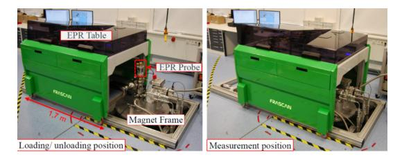
Fig. 4.1: The photograph of FRaSCAN EPR spectrometer in position for loading/unloading of the probe and measurement position. The picture was taken in June 2020.
