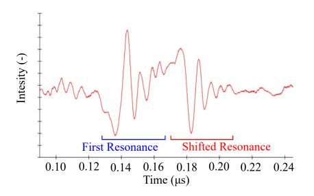
Fig. 6.7: Rapid scan measurement of 2mM BDPA dissolved in toluene. The notdegassed sample ( $\approx 50$  nl) was sealed in LSH. The parameters of the measurements: frequency generated by AWG at 390 GHz in chirp pulses of 1.8 GHz (V Shape), sweep rate 0.5  $\mu$ s, T=293 K,  $B_0 \approx 14$  T, number of averages = 2 000 000.
