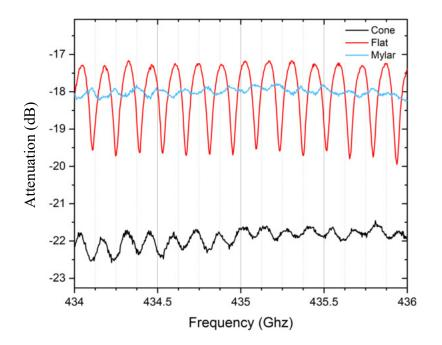
Fig. 4.24: VNA measurement of different EPR probe windows. A different standing wave intensity is observed with a similar pattern for each of the tested windows: conycal (teflon), flat (teflon) and PET (Mylar).
