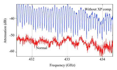
Fig. 4.14: Red) The measurement with the last Faraday Rotator and wire grid polarizer. Blue) The measurement without first the Faraday Rotator and wire grid polarizer in front of XP mixer.
