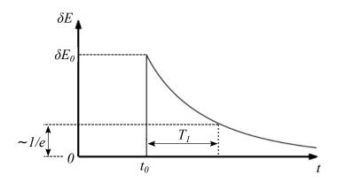
Fig. 2.6: Decay of the extra energy  $\delta E_0$  in the system at the time  $t_0$  to 1/e value. The relaxation time  $T_1$  is an indirect measurement of the coupling between the spin system and its surroundings.
