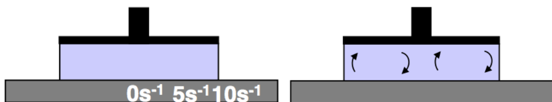
Obr. 7 Schéma geometrie deska–deska [2]
