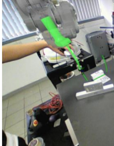
Figure 2.1: Physical handheld pointer used as position target for the end effector used in the work by Ong et al. [11].
