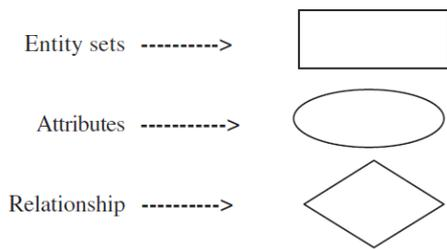
*Figure 7: Shapes used in Entity-Relationship Diagram*
