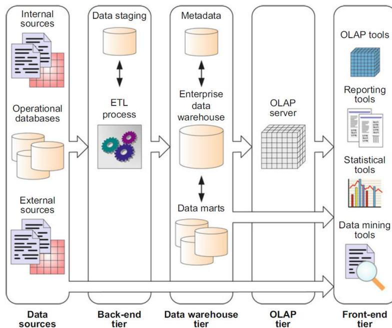
Figure 13: Typical data warehouse architecture
