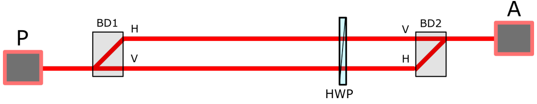
Figure 26: Scheme of the polarization Mach-Zehnder interferometer: beam displacer (BD), half wave plate (HWP), polarization state preparation (P), polarization state analysis (A). The separation between the two paths is 4 mm.
