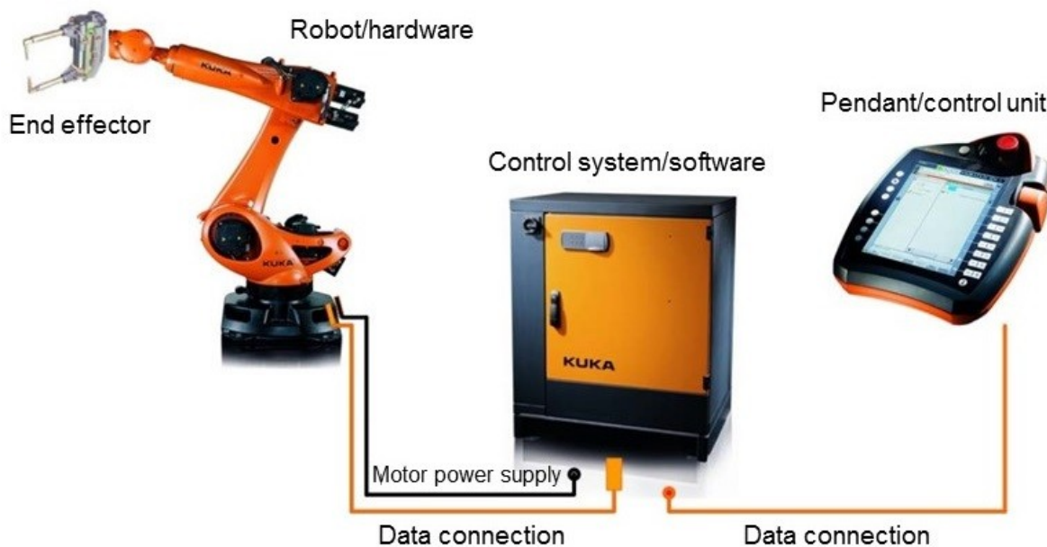
Fig.11 Example of a typical structure of an industrial robot composed of hardware, software and a control unit [9].
