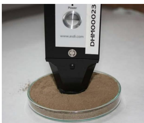
Obr. 5 The ASD High Intensity Contact Probe
