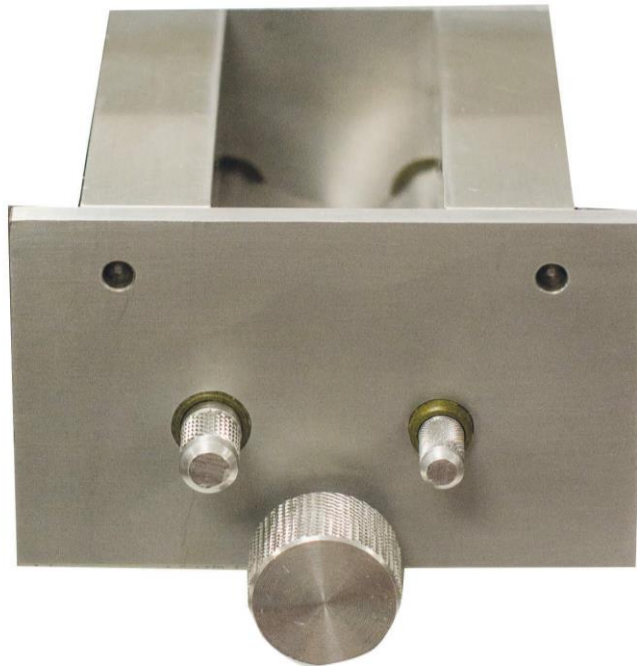
Figure 4: Mixing bowl of Mixolab 2 [64]
