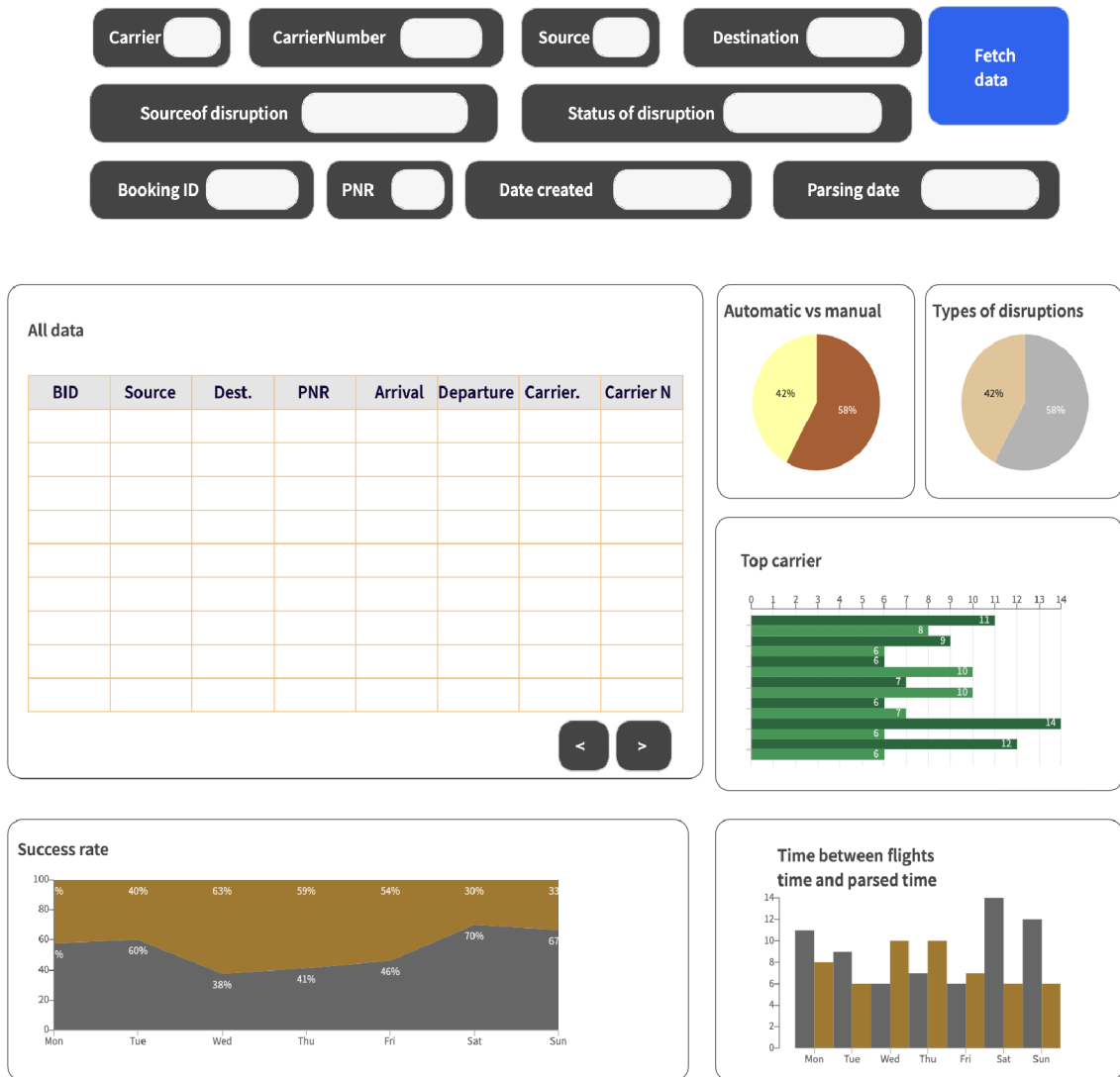
Figure 5.2: Mock-up of web application. Figure shows a mock-up of a web application with all its components. There is a filters section at the top, and beneath, there is a table of all fetched data. On the sides, we can see graphs that depict the statistical analysis of fetched data and its visualisation.
