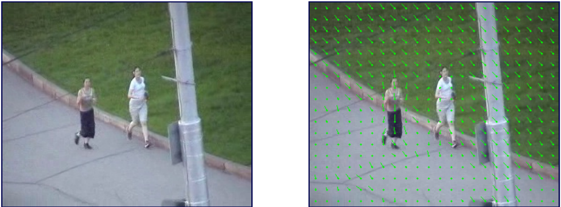
Figure 2.10: Illustration of the optical flow. On the left there is one frame (out of the pair) and on the right there is visualized optical flow (subsamped).
