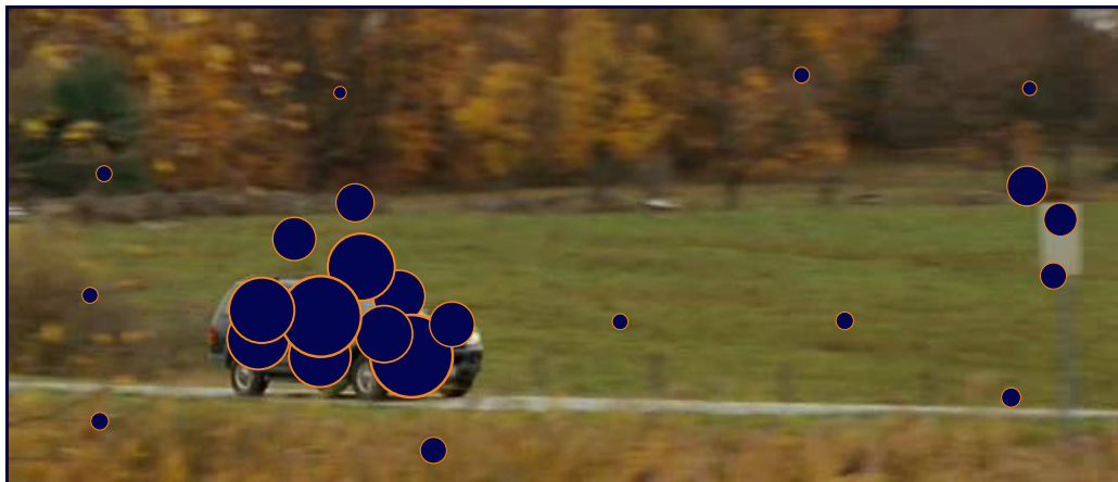
Figure 2.13: Illustration of the particle filter. The particles (blue dots) represent expected positions and their size is proportional to their weight. As can be seen, the most particles are concentrated around the most expected position, while only a few cover the rest of a space.
