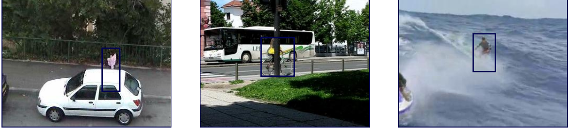
Figure 2.14: The partial occlusion. The objects are partially hidden, yet we want to track them.
