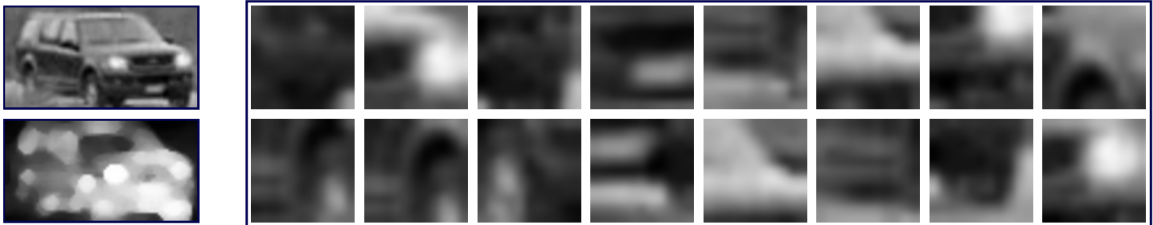
Figure 4.2: Results of Monte Carlo Points To Track Generation. On the left side there is the original bounding box with its mask. On the right there is a set of enlarged points in their neighborhood as they are supposed to be used in tracking. It can be seen that some of them are duplicated as well as barely unique. The computational time was disproportionately long due the number of missed generations.
