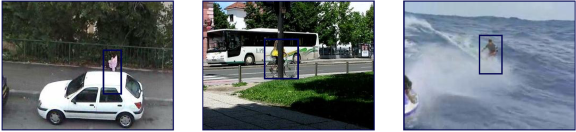
Figure 2.14: The partial occlusion. The objects are partially hidden, yet we want to track them.
