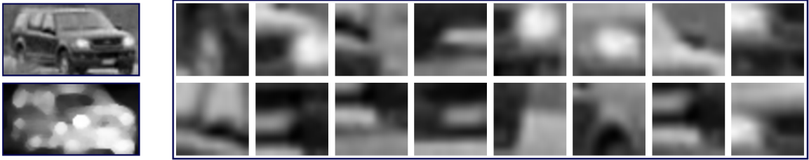
Figure 4.3: Results of GFTT Points To Track Generation. On the left side there is the original bounding box with its mask again and on the right there are enlarged points in their neighborhood generated by this method. It can be seen that the quality increased.
