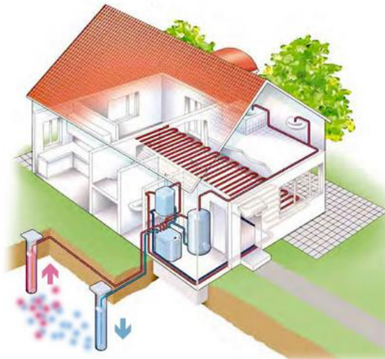
Figure 11-water to water heat pump[11]
