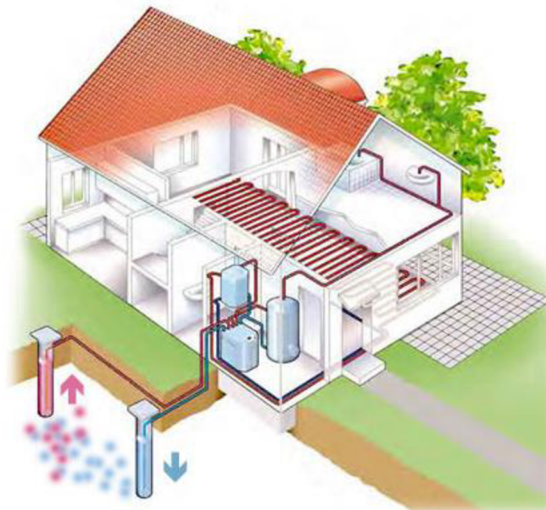
Figure 11-water to water heat pump[11]
