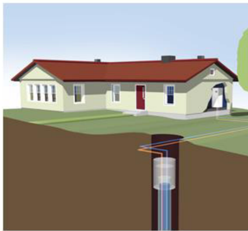
Figure 9-heat pump ground to water with boreholes[14]
