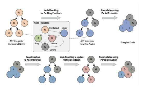
Figure 4.6: Node optimization and deoptimization in Truffle<sup>6</sup>
