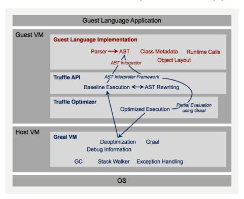
Figure 4.4: Architecture of a Truffle language, arrows denote program execution flow<sup>4</sup>
