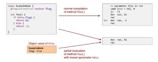
Figure 4.1: Partial evaluation with constant folding<sup>1</sup>
