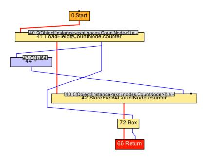
Figure 4.3: Graal program graph, visualized using IGV<sup>3</sup>
