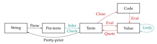
Figure 4.8: Data flow overview. Cyan is elaboration, red normalization-by-evaluation
