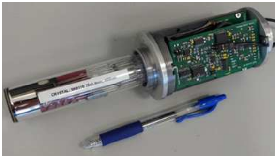
Fig. 10. The final look of the IND system (without housing), compared to a pen
