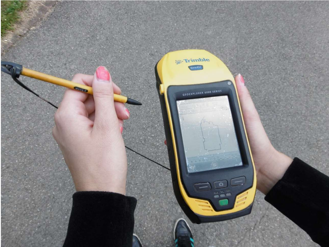
Figure 4: GPS mapping process of the parking lot with GeoExplorer device
