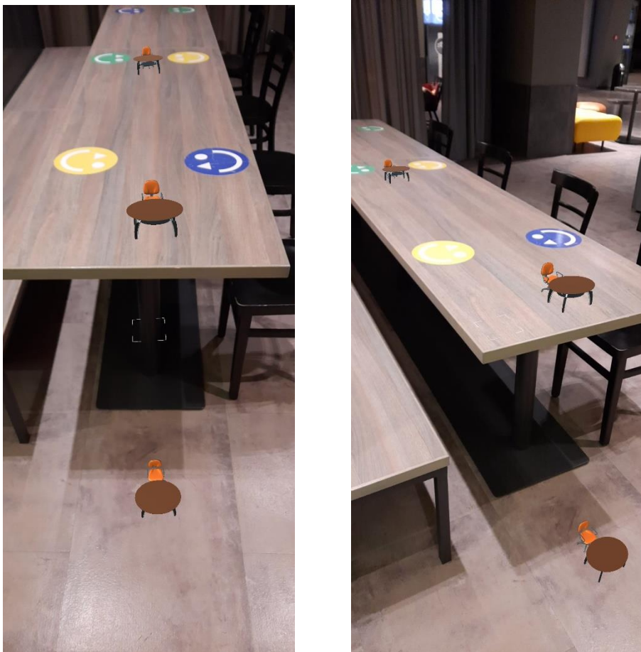
Figure 15. An example of SLAM ground detection
