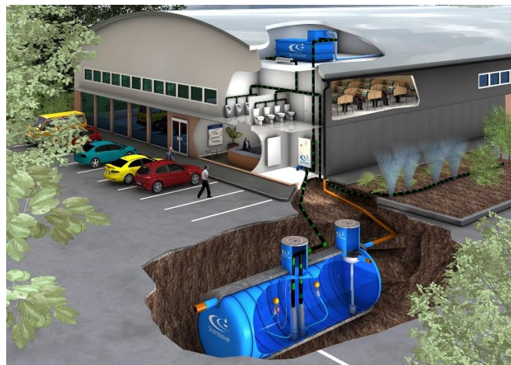
Fig. 38.: Utilization of rainwater – the picture represents utilization of water for irrigation, flushing toilets or washing (Designed by Stomrsave Ltd.)
