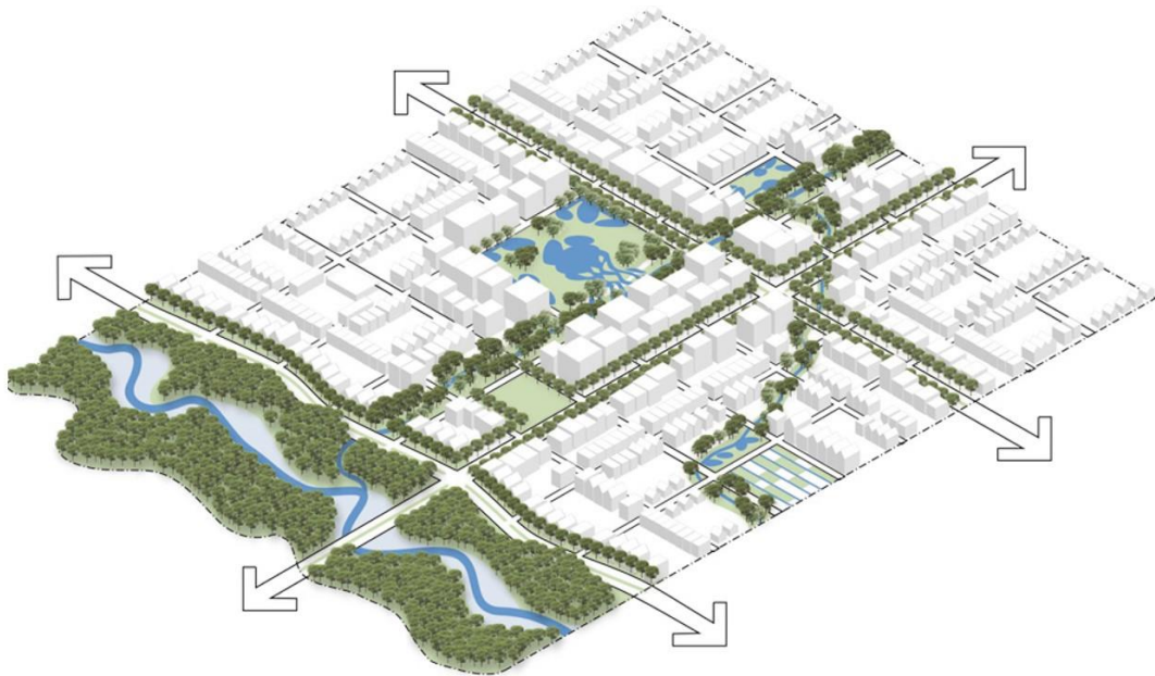
Fig. 9: Diagram of the using “slow, spread, soak” techniques - Instead of using conventional approach (drain, direct, dispatch), a decentralized approach can be applied, where complex stormwater infrastructure can positively influence a hydrologic regime by using “slow, spread, soak” techniques that infiltrate, filter, store, and evaporate stormwater runoff (Reference - University of Arkansas Community Design Center; 2010)
