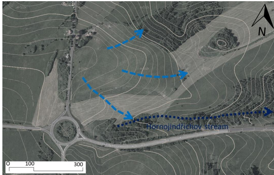
Fig. 42 – Diagram of the topography at the site with 2 meters contour lines - This diagram represents a topography at the site with 2 meters contour lines. This diagram help visualizes natural stormwater runoff based on the typography, including Hornojindřichov stream in the bottom of the site (Created by Author, original data are from Geoportal, 2015)
