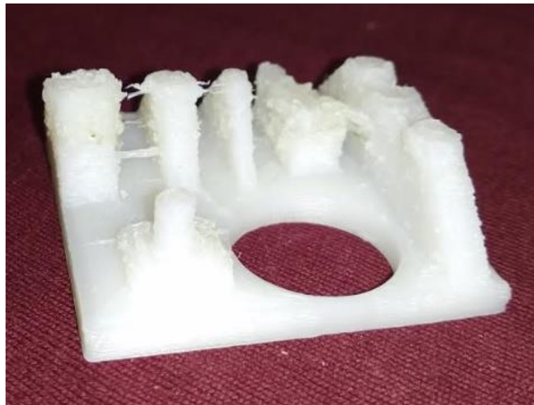
Figure 16 - defects in Printed part
