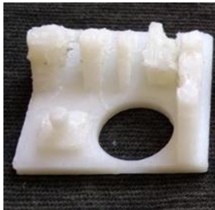
Figure 11 - Defects in printed part - HIPS
