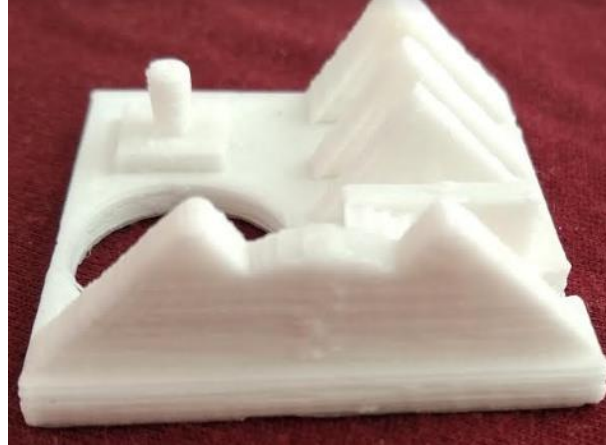
Figure 31 - Printed part with bad surface
