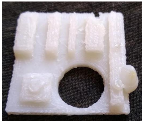
Figure 13 - Defects in printed part
