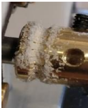
Figure 30 - Materials stick in feeder
