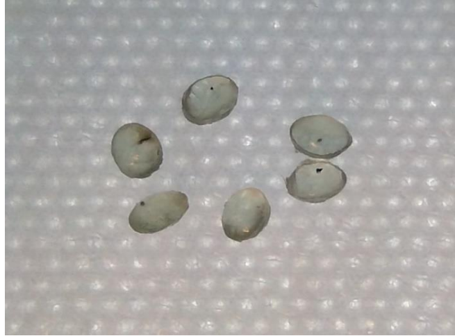
Figure 9: Black spots in amorphous PET pellets. Source: own source.
