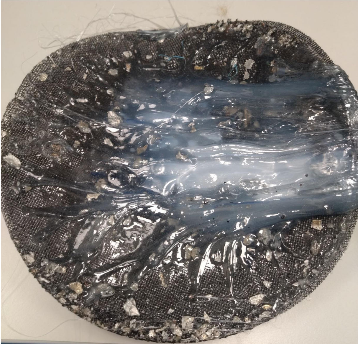
Figure 10: Used filtration screen covered with aluminium and metal as well as some charred particles. Source: own source.
