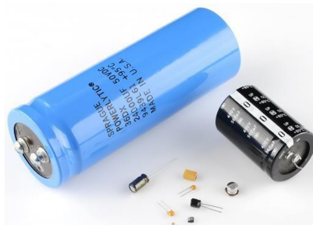
Figure 23 Sizes of Capacitors [22]
