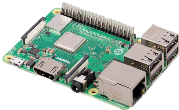
Obr. 3: RaspberryPi model 3 B+[8]
