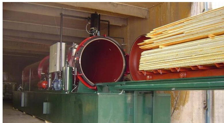
Figure 3 Charging the timber to the vessel of vacuum pressure impregnation plant ( http://www.wtt.dk/products/impregnation/impregnation-plant/pictures )
