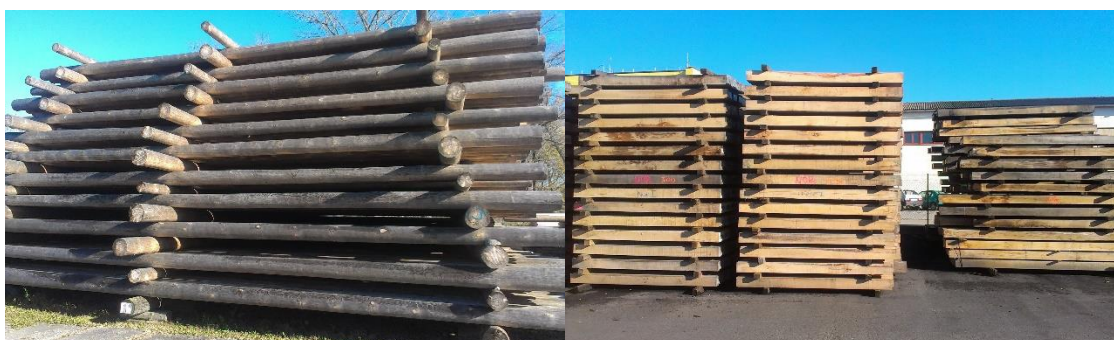
Figure 1 The storage of air-drying poles (left) and railway sleepers (right) (unpublished, photo was taken in the company Impregnace Soběslav).
