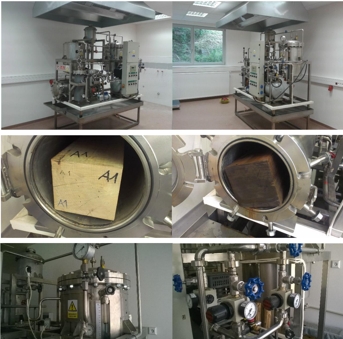
Figure 12 Laboratory vacuum - pressure plant, basic view (upper); vessel with untreated and treated sample (middle); preheater and tubes with valves (bottom)
