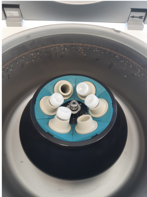
Figure 7: centrifuge containing yogurt tubes for syneresis analysis.
