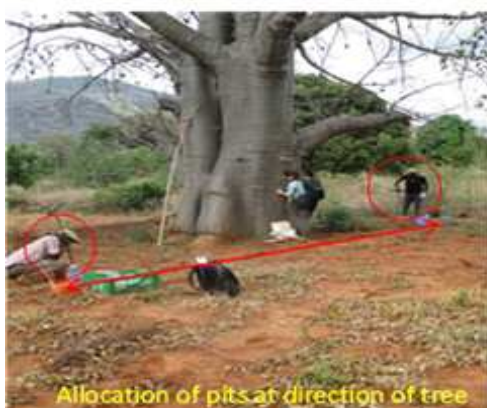
Figure 7. Soil sampling - allocation of the pits at opposite directions of tree trunk and at half distance between the trunk and crown limit.
