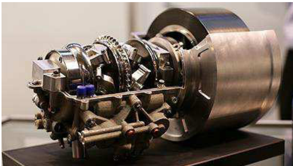
Obr.5 KERS s prevodovkou Torotrak v reze [9]
