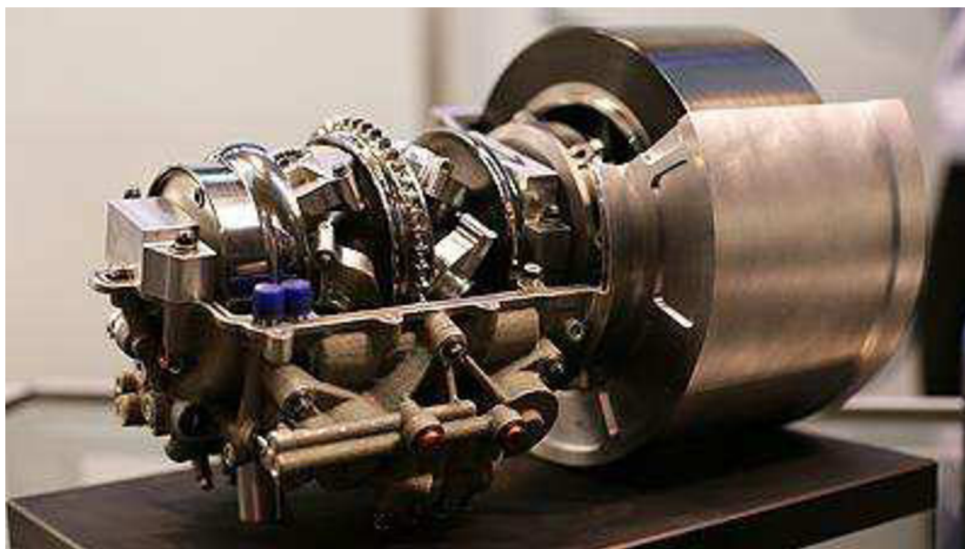
Obr.5 KERS s prevodovkou Torotrak v reze [9]
