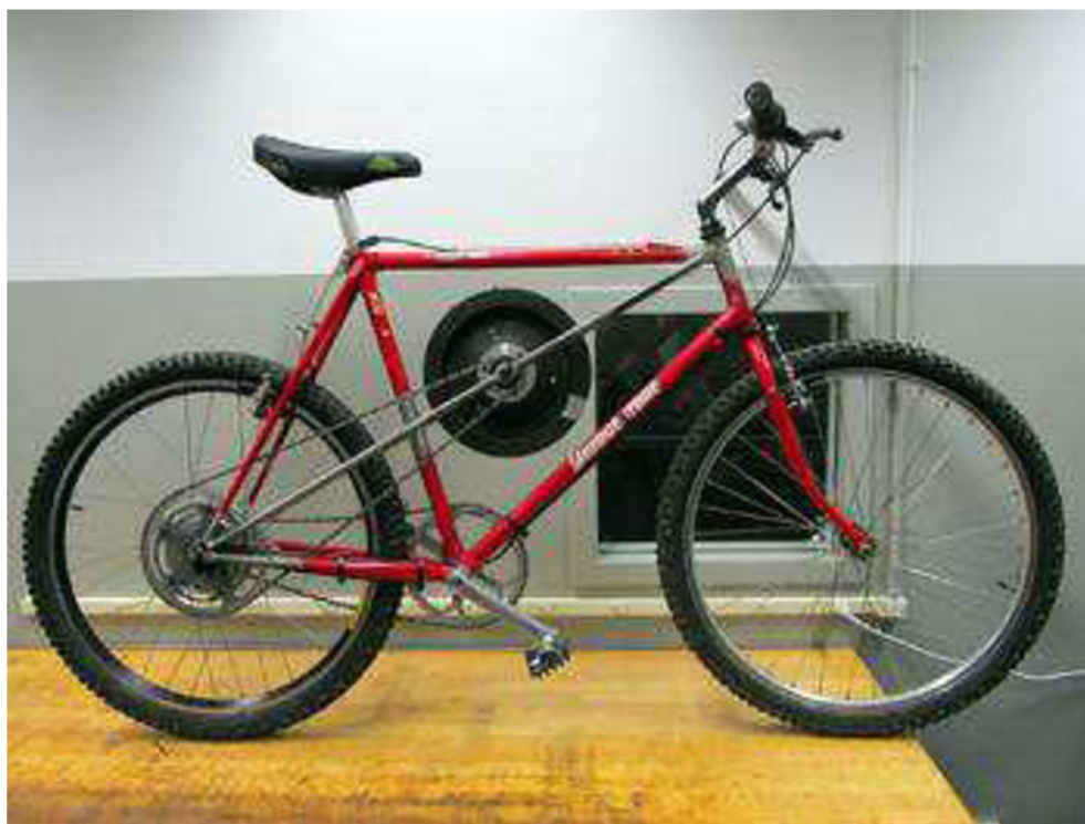
Obr.7 Flywheel bicycle od Maxwella von Steina [15]
