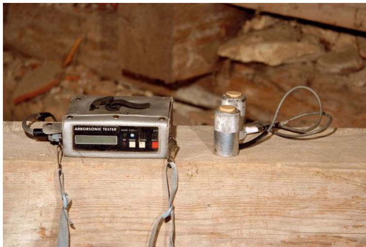
Obr. 13 Arborsonic Decay Detector
