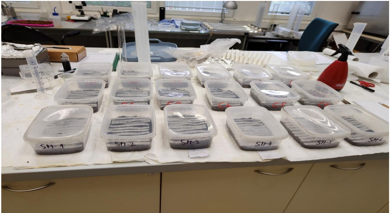
Figure 10. Experimental boxes made airtight to assume 100% humidity
