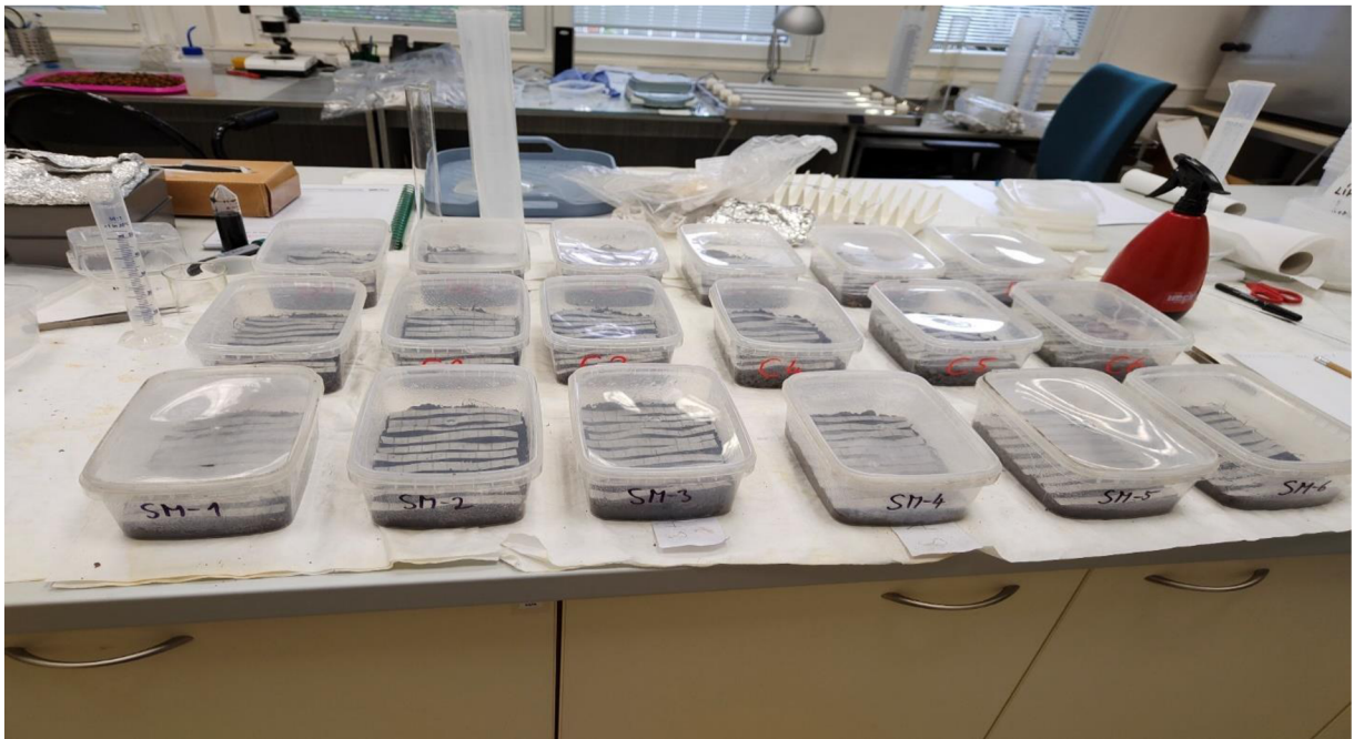
Figure 10. Experimental boxes made airtight to assume 100% humidity
