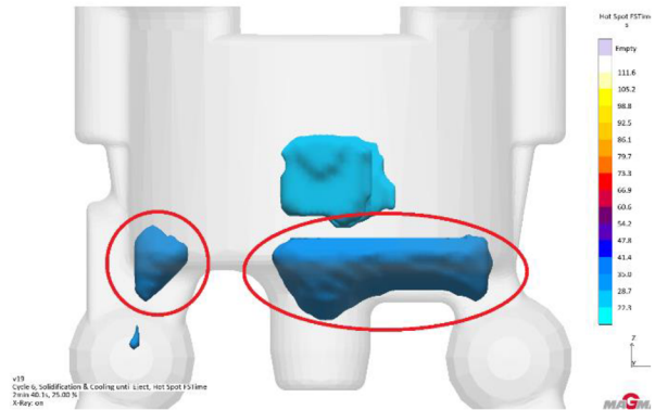
Obr. 3-29 Hot Spot v oblasti 3
