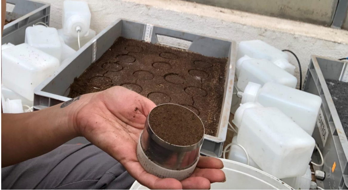
Fig. S3. Undisturbed soil samples collected from the upper 10 cm thick layer of each box using standard stainless-steel soil sample rings.
