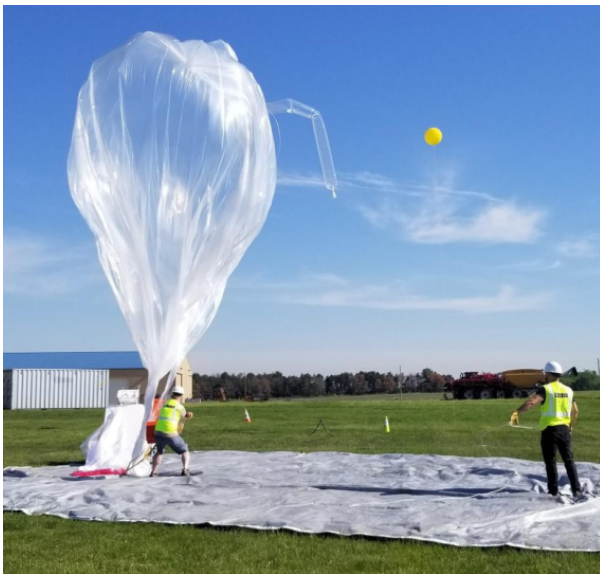
Fig. 1.5: Zero-pressure balloon, adapted from [7].
